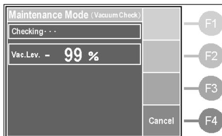
When the check is done, depending on the result the screens shown below will be displayed. If it is NG, check if the altitude setting is set correctly in default set mode (→P20). If the cause might be due to moisture, run the “Unloaded Muffle Firing” (→P7) and check one more time. Press the “Back” button to move to maintenance mode.
