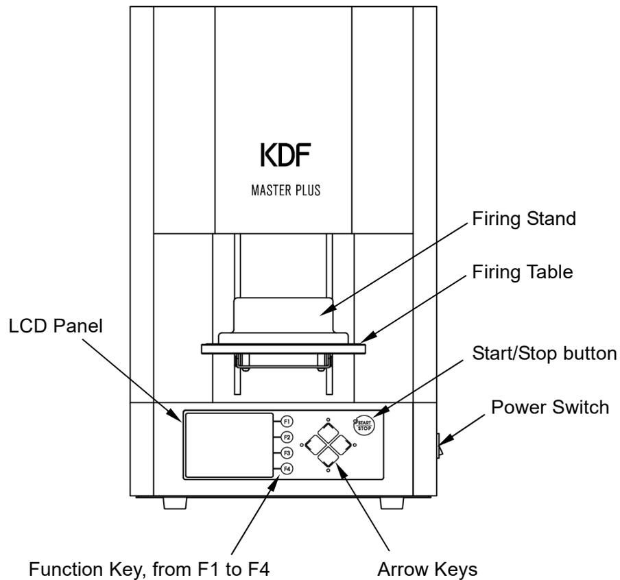
Firing Stand : A firing stand used to place the firing tray and firing objects.
