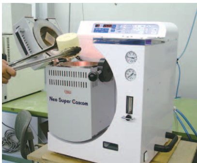
Place a burned out casting ring
