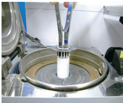
Insert the Crucible in the Muffle
