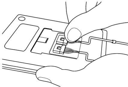
4 Insert the grip cords into the grooves of the frame to put back the cover in place.
