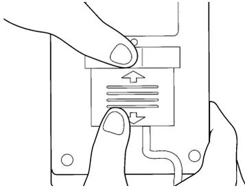
2 Hook the remover provided to the cord connector to pull out.
