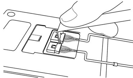
3 Plug a new grip cord connector with the red mark upside to insert completely.
